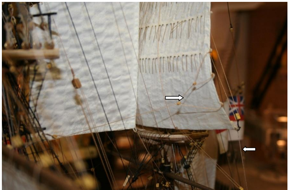
23.18 Mizzen topsail bowlines and bridles The bowlines lead forward, cross and seize to the aftermost main shroud then down to belay on the quarterdeck. The mizzen topsail sheet lines (lower right) is attached to the corner clueline cringle and reeves down to the cross jack to belay on deck.
