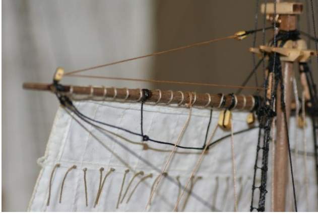
19.2 Mizzen topsail yard horses and stirrups The first item on the yard is the horses and stirrups. I installed two per side the same as the fore and main topsail yards.
