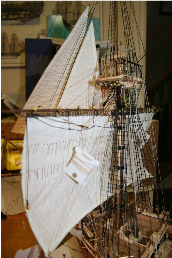
22.14 Fore course cluelines The cluelines, bunt lines and leech lines were all installed prior to crossing the yard to the mast.
