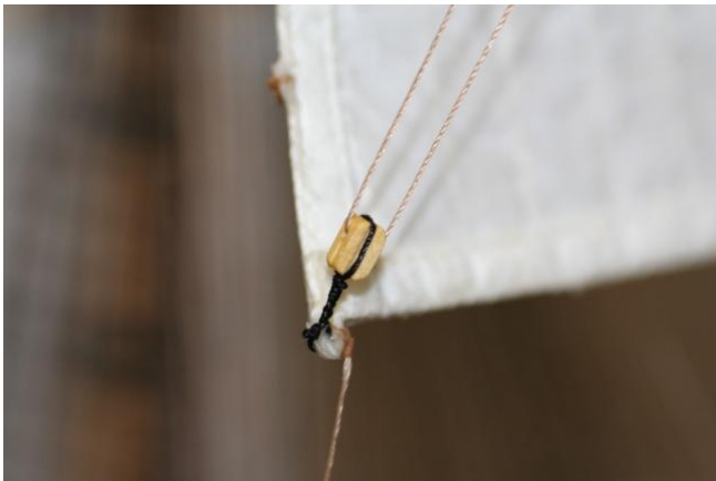
19.4 Mizzen topsail yard clueline blocks Two clueline blocks are stropped and attached on the inboard side of the first quarter of the yard. Two other blocks are attached to the clueline cringle on the bottom corners of the sail.
